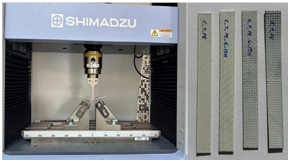
Figure 12. Flexure test and specimens
